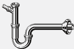
Pipe odour trap Plus siphon - chrome-plated brass Components screw fitting G¾, closing panel, adjusting pipe 200 mm, outlet elbow 220 mm quality controlled in accordance with EN 274 Model 5611.6
